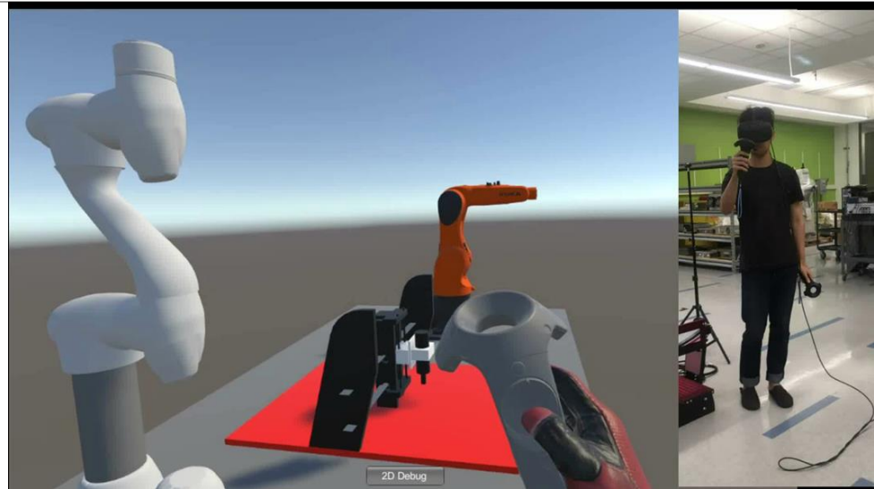
Figure 7. The digital twin generation: use of VR headset for real-time interaction with physical machines via digital twins
